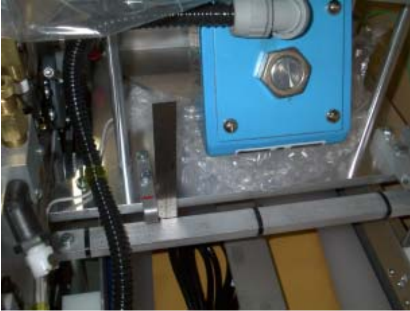
Padding to support the weight of the control box is important.
