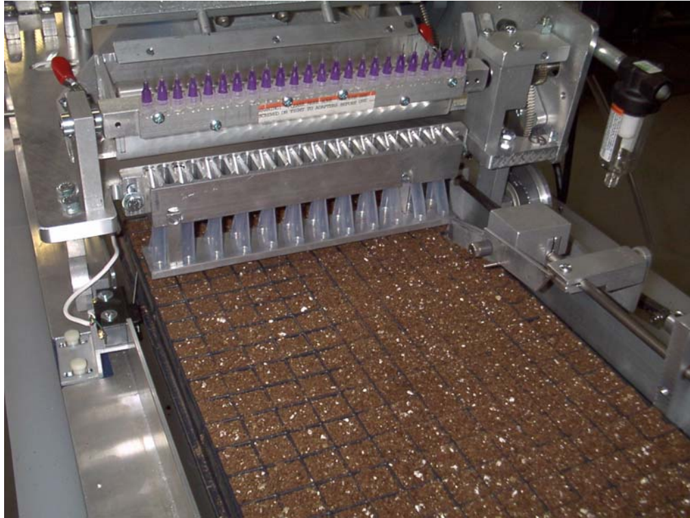
Double row drop tube sows two rows of seeds per cycle.
